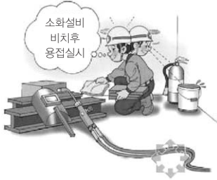
소화설비 비치 후 용접 실시 (sohwaseolbi bichi hu yeongjeop silsi) Welding after installing firefighting facilities
